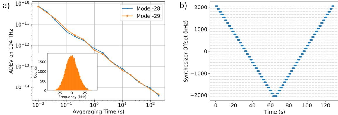
**Figure 2:** (a) Overlapping Allan deviation and histogram counts of the synthesized frequency at 2 adjacent silica comb lines (mode number referenced from the pump laser). (b) Arbitrary laser frequency control across 32 levels by digitally tuning the offset phase lock. Counter trace for 100 ms gate/2 s pause per level is in blue. expected synthesizer frequency levels are in dotted gray.
