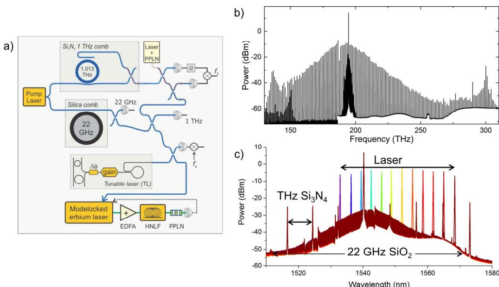
Figure 1: (a) The frequency stabilized dual-Kerr microcomb and integrated Vernier tunable laser optical synthesizer, including reference mode-locked laser supercontinuum. (b) The octave spanning 1.013 THz  $\text{Si}_3\text{N}_4$  and tightly spaced 22 GHz silica microcombs provide full stabilization to an RF clock, while (c) the III/V-Si based integrated tunable laser allows for ultra-stable synthesis at arbitrary optical frequencies across the laser tuning range.
